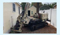
Our Drilling Crew's expertise was put to the test maneuvering the GeoProbe® rig to collect soil, soil vapor and groundwater samples as well as monitoring well installs at various types of job sites over the summer.
