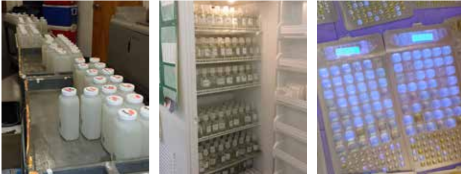
Pictured from L to R: A single day "event" of BOD samples ready to be wheeled into the lab. Space is a premium in a BOD incubator. Samples fluoresce under a black light indicating the presence of E.coli .
